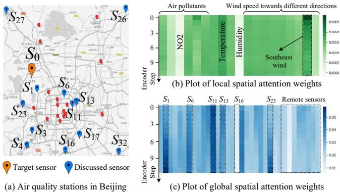
Figure 5: (a) The distribution of air quality sensors throughout Beijing, where  $S_0$  is the target sensor we discuss. (b)-(c) The attention matrix obtained from the local and global spatial attention mechanisms, where each row is the attention vector over the inputs.
